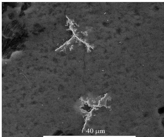
**Figure 5 – The threadlike branchy secretions of gold in the limonite. Polished section 3. The picture is executed on JXA microprobe – 733**
