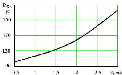
**Figure 3 - The dependence of the total resistance  $R_x$  opener on the speed  $v$**
