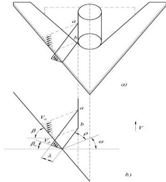
**Figure 4 - The working body of the opener (a) and the design scheme, the forces acting on side opener (b)**
