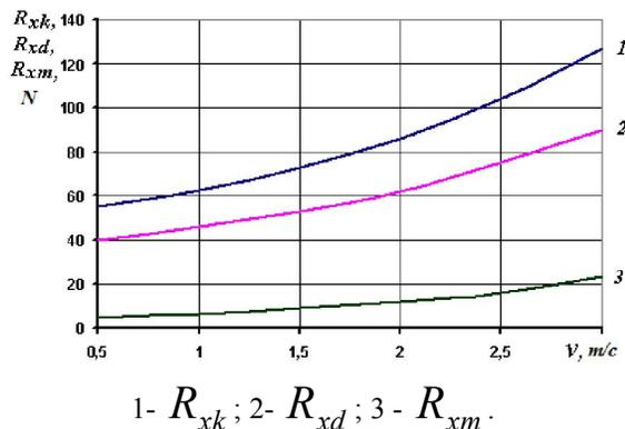
**Figure 5 – Dependences of the components of ploughshare traction resistance**
