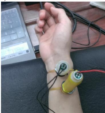
Figure 2. The actual measurement setup. Both two detectors are attached on the wrist.
