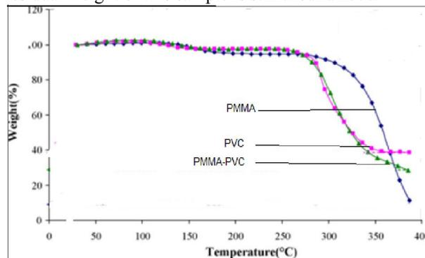
Figure (3.2 a): TGA thermograms of PVC, PMMA and PVC/PMMA.
