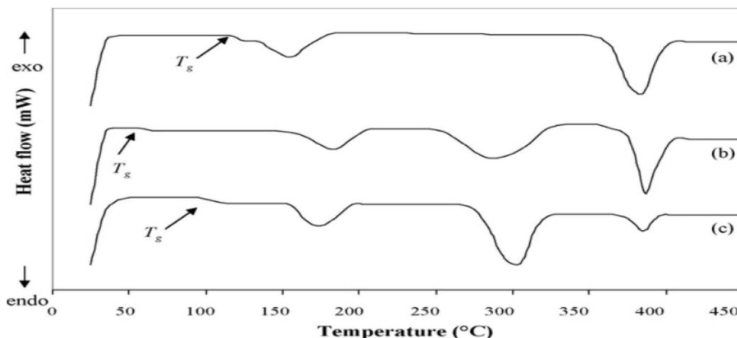
Figure (3.1a): DSC thermograms of (a) pure PMMA, (b) pure PVC and (c) PMMA-PVC.
