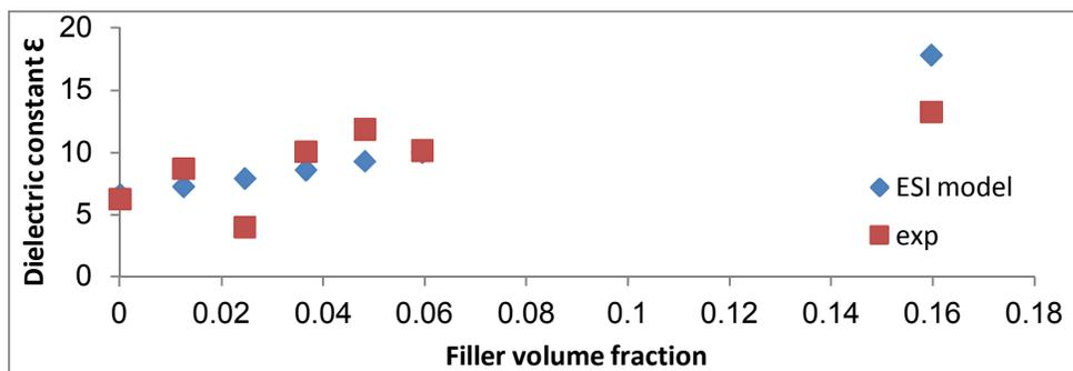
Figure (3.6): Relation between the dielectric constant and the filler volume fraction for all samples.
