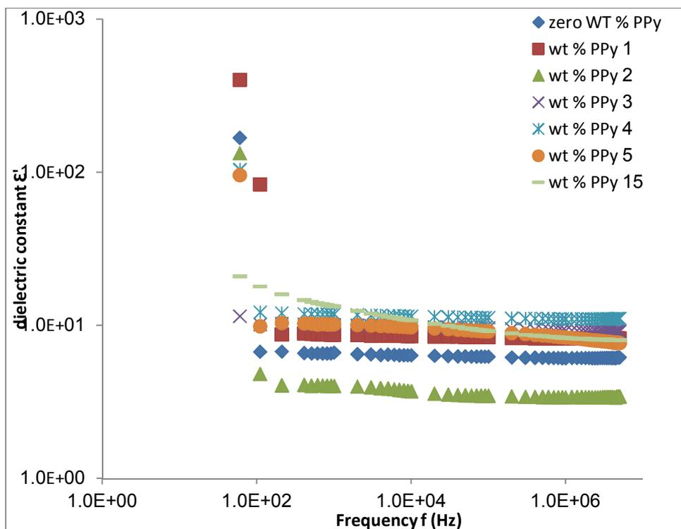
Figure (3.5): The relation between the logarithm of dielectric constant and the logarithmic frequency for all samples.
