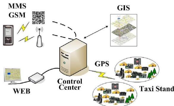
Figure 1. The Framework of the Dispatching System
