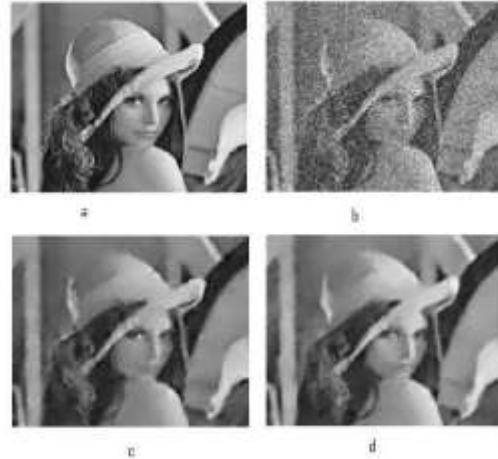
Fig. 2 The original image in a, the image with additive noise in b, the denoised image by using ICA_DL in c, and the denoised image by using k_SVD in d.
