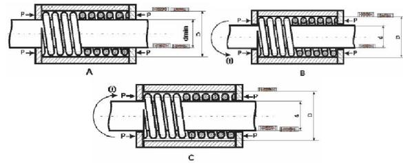
**Fig. 1. The fit scheme on the working surfaces of the hinge bearing with elastic spring insert: A - bearing is at rest; B and C - the axis rotation (spigot) in different directions**
