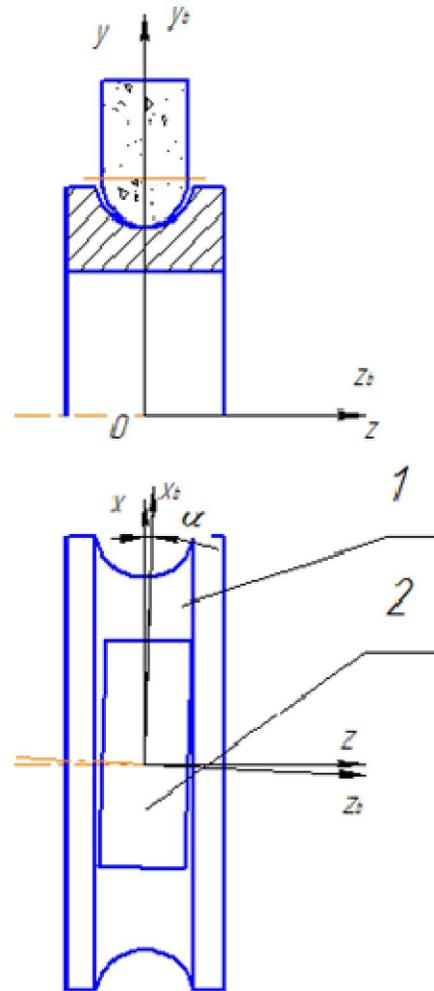
**Fig. 3.** The scheme of blank-1 and sharpening stone arrangement -2
