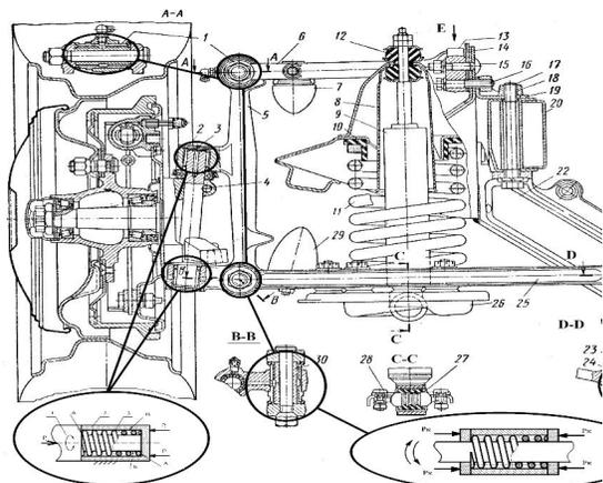
**Fig. 2. Front suspension of vehicles with possible options of replace the existing hinges knots with the assemblies of new design**
