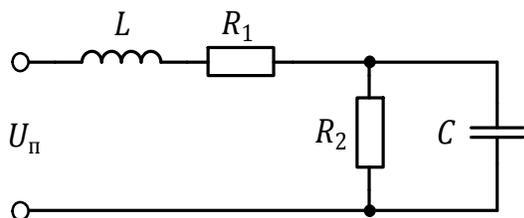
**Fig.4. Equivalent Circuit of the Current Regulator Load Substitution.**
