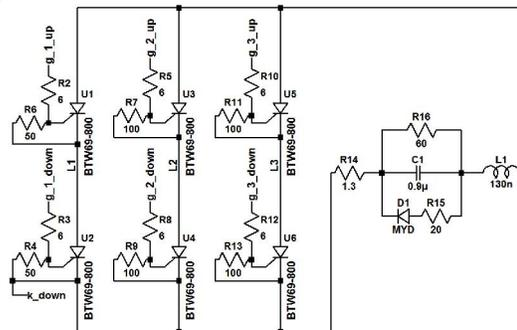
**Fig. 6. Model of the Power Module of the Thyristor Current Regulator**
