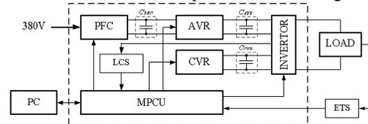
**Fig. 9. Unit Block Diagram for MAO with Transistor Current Regulator**
