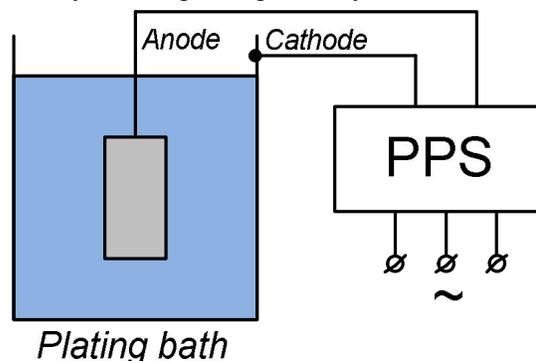
**Fig. 1 – Unit Block Diagram for the Microarc Oxidation.**
