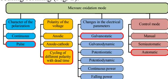
**Fig. 1 – Classification of the Microarc Oxidation Modes**
