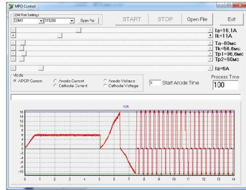
**Fig. 8. Interface of the Current Regulator Control Program for MAO**
