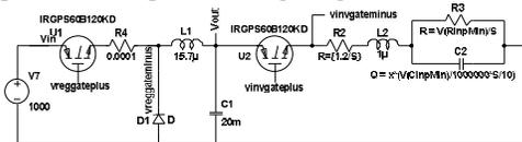
**Fig. 11. Integrated Model of the Transistor Current Regulator for the MAO Devices**
