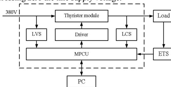
**Fig. 5. Thyristor PPS Block Diagram**
