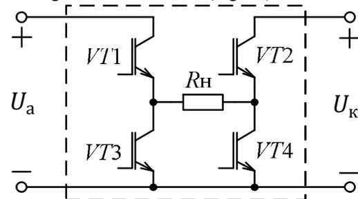
**Fig. 10. Conceptual Voltage Inverter Diagram**
