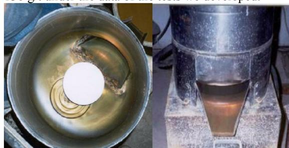
**Fig. 8. Gilt bowls of the concentrator after receiving the concentrate from ore Vein No 14 of Arkharly field (top and front views)**
