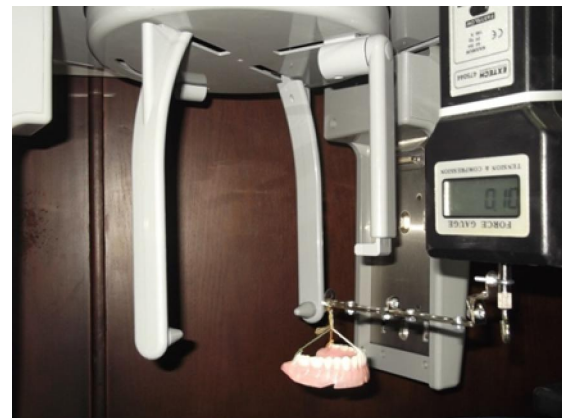
Figure 1. The denture suspended, in a zero tilt, to the rigid extension arm which is attached at right angle to the sensing head.
