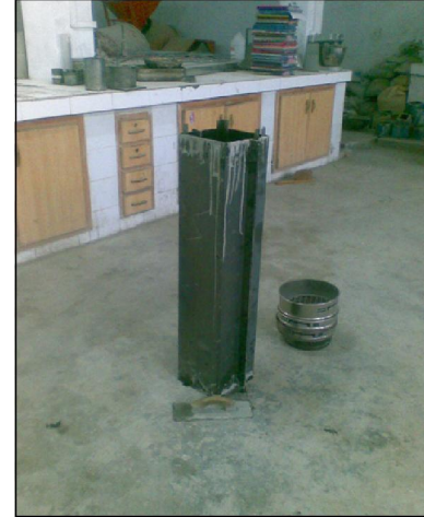
Fig.2 Steel plates formwork for casting concrete columns
