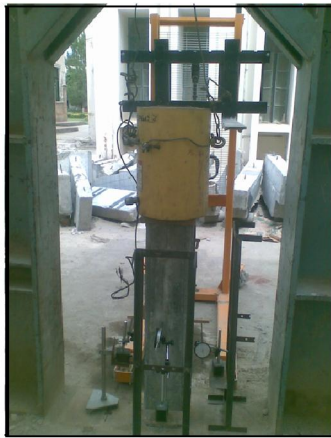
Fig.8 Arrangement of specimens for axial load testing
