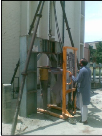
Fig.7 Placement of specimen for axial load testing
