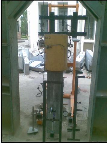
**Fig.9** Arrangement of dial gauges to measure the deformation
