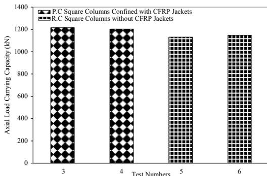
**Fig.13** Strength comparison of confined P.C & unconfined R.C columns
