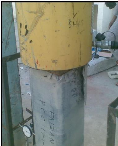
**Fig.11** Failure mode of CFRP confined column
