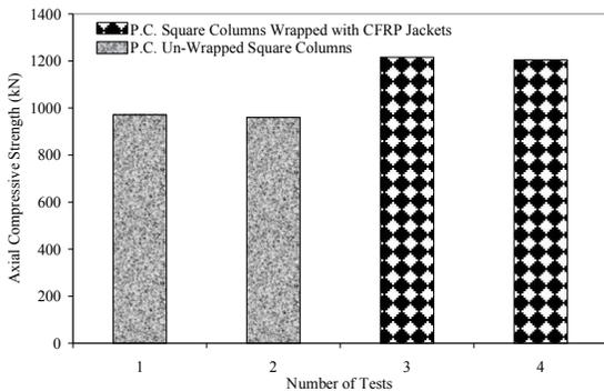
**Fig.12** Strength Comparison of unconfined & confined P.C columns
