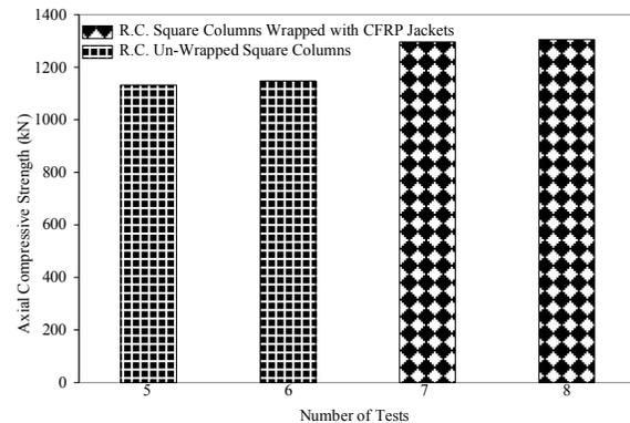
**Fig.14** Strength Comparison of unconfined & confined R.C columns
