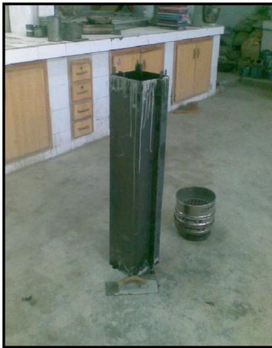
**Fig.2** Steel mould for casting of concrete columns
