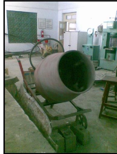
**Fig.4** Concrete mixer for preparation of specimens
