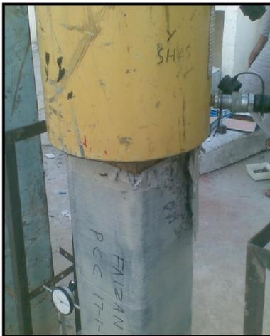
**Fig.11** Failure mode of CFRP confined column
