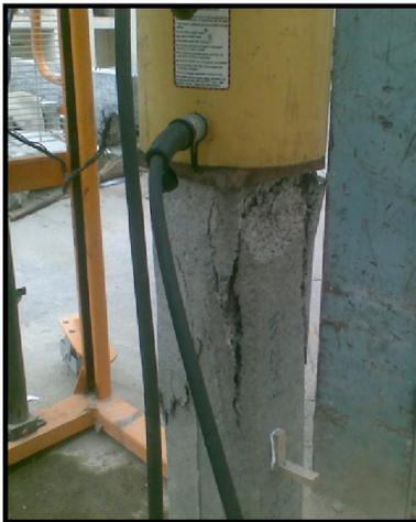
**Fig.10** Failure mode of un-confined concrete column
