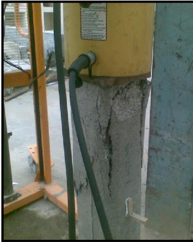
**Fig.10** Failure mode of un-confined concrete column
