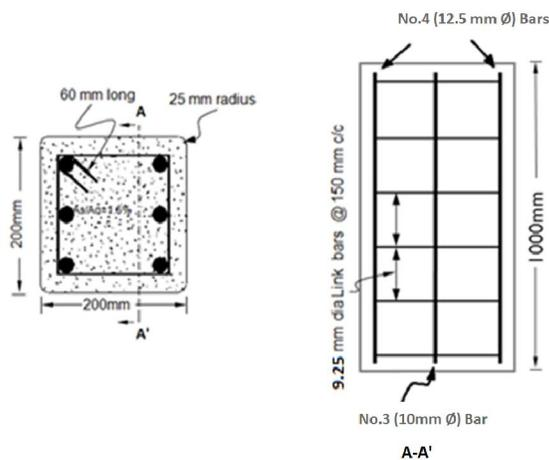
**Fig. 1.** Steel reinforcement bars arrangement in square concrete columns.
