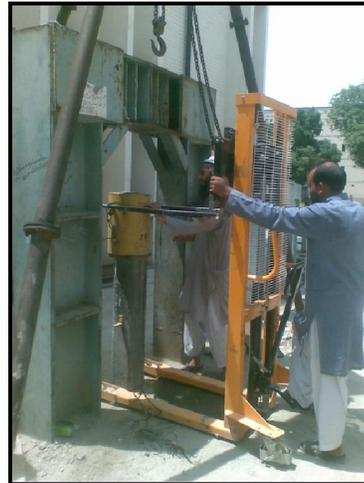
**Fig.8** Arrangement of concrete column in axial load test up
