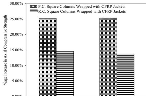
**Fig.15** Strength comparison of confined P.C & R.C columns
