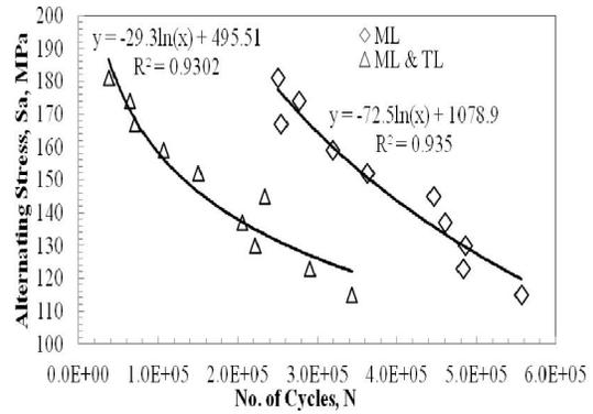
Figure3 (S-N Curves of constant amplitude)
