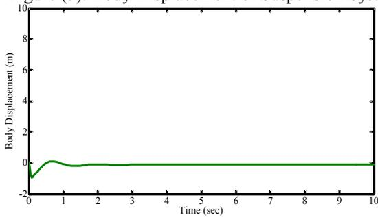
Figure (6): Body Displacement variations for LQR Controller
