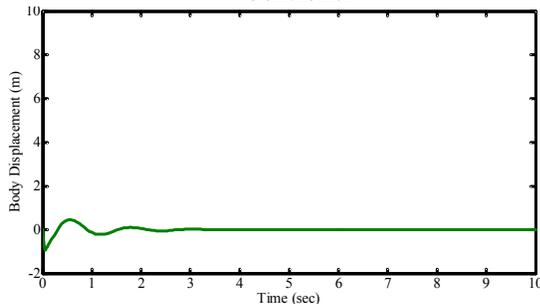
Figure (7): Body Displacement variations for Optimal Control Integration based Intelligent Controller
