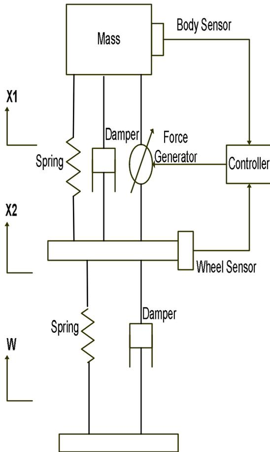
Figure (1): Active Suspension using Quarter Vehicle Model
