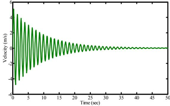
Figure (10): Velocity Variations of Suspension System
