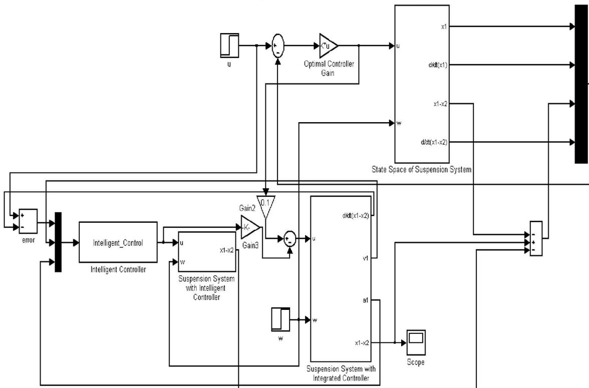
Figure (4): Active Suspension using Optimal Control based Intelligent Controller SIMULINK model
