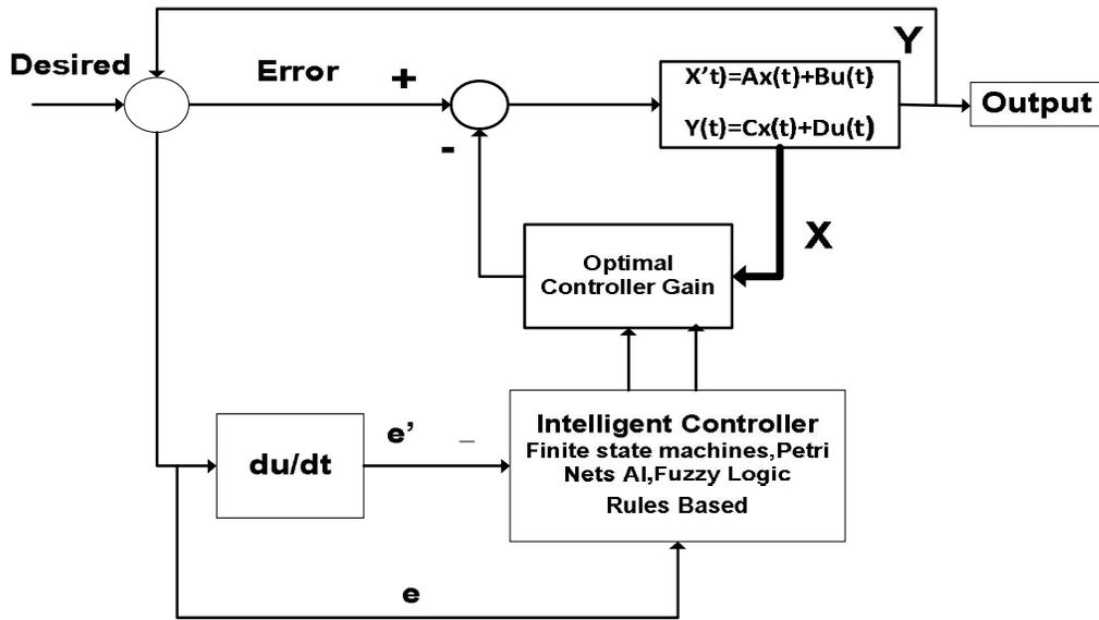
Figure (3): General Layout of Optimal Controller based Intelligent Controller
