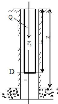
**Fig.1** Scheme of the descent in to the well drilling tools
