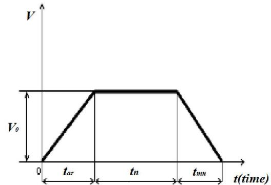
**Fig.2** Changes in velocity  $V$  drilling tools from time when running in hole.
