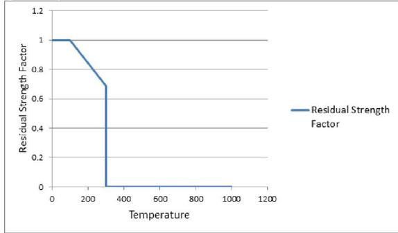
Figure 1: Residual compressive strength of concrete after cooling.
