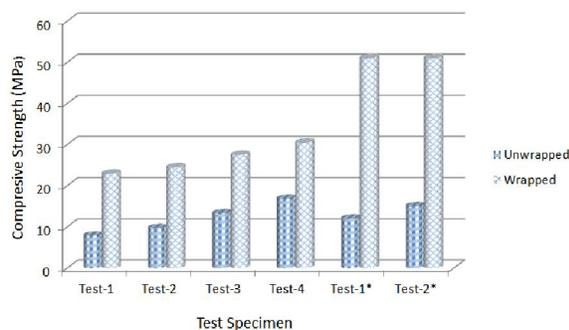
Figure 2: Comparison of unheated experimental work versus post heated published data\* for low strength concrete
