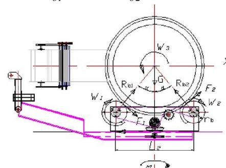
**Fig. 4. Bale rotation about the longitudinal axis Oz**
