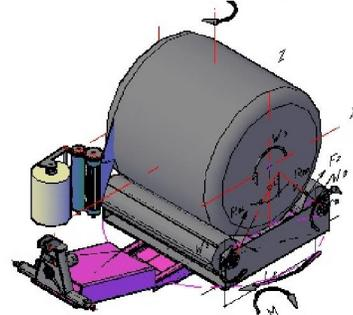
Fig. 2. Wrapper – mechanical-mathematical model
