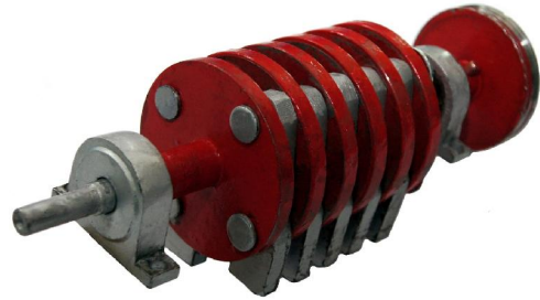
Fig. 1: Working element of an ice-breaking machine. Visible steel hammers (grey) loosely axled between disks (red), which in turn are mounted on a common shaft.
