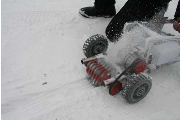
Fig. 6: Snow-ice chipping process
