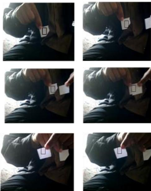
Figure6, Video 2;90 frames, target model fully occluded with other object of same appearance and shape, applied to traditional meanshift algorithm
