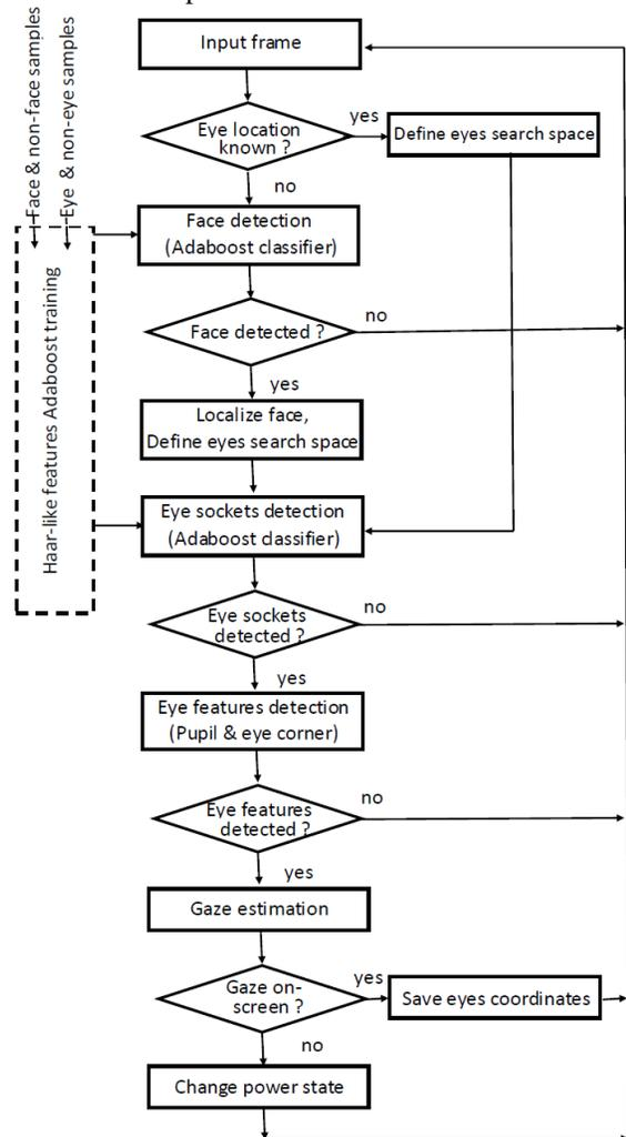
**Figure 7. Eye Gaze Tracking Algorithm.**
