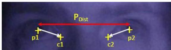
**Figure 6. Eye feature vector determination.**
