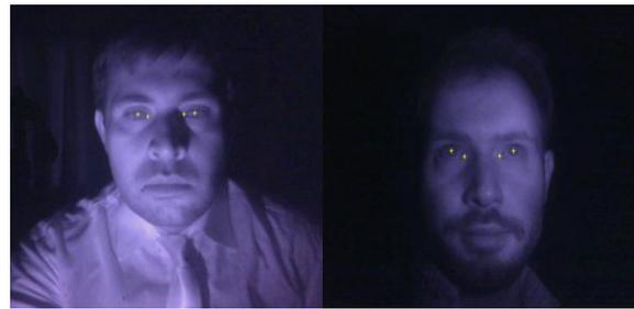
**Figure 8. Output from the proposed system depicting successful pupil centers and inner eye corners detection.**
