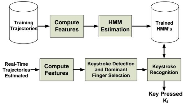
Fig. 8. Keystroke Detection and Recognition Algorithm
