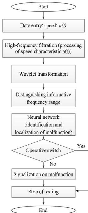
**Fig. 1 – Algorithm of NN diagnostics using wavelet analysis and neural network.**
