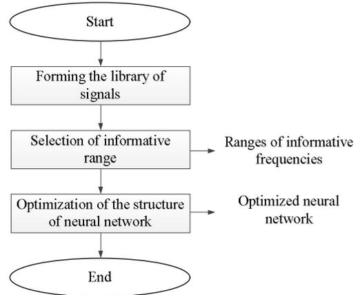
**Fig. 2 – The algorithm for preparing the diagnostic system.**
