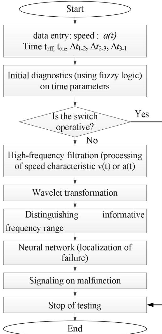
**Fig. 3 A two-step algorithm of NN diagnostics using fuzzy model and neural network.**
