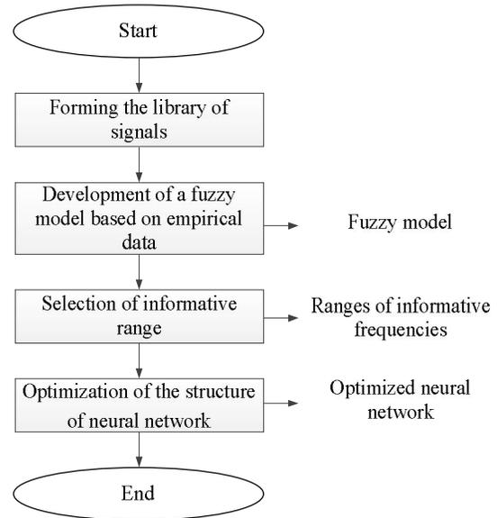
**Fig. 4 The algorithm for preparing the diagnostic system on a two-step algorithm.**
