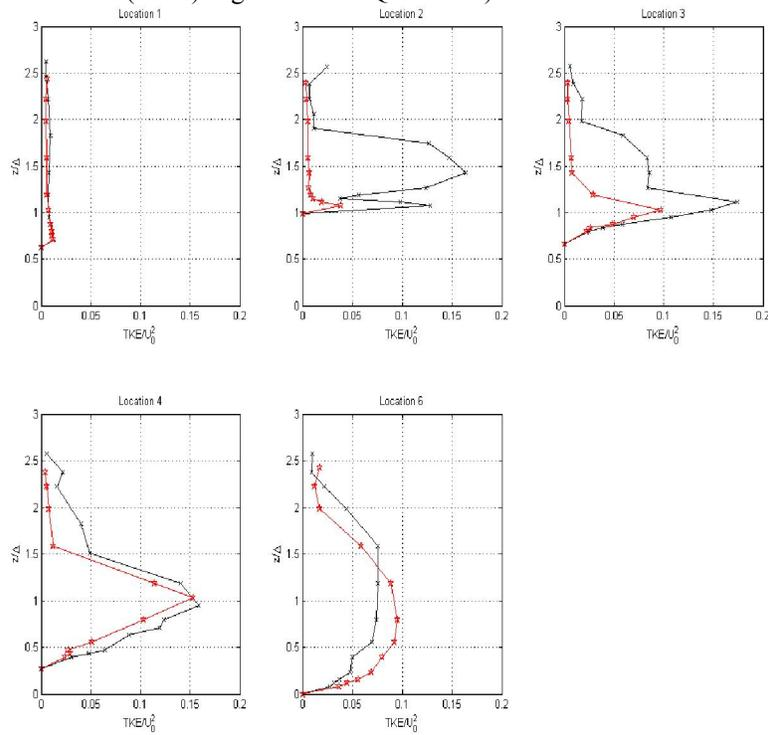
Figure 3. Comparison of turbulent kinetic energy at different locations for the vegetated and non-vegetated weir (\* (red) non-vegetated weir and x (black) vegetated weir  $Q=40$  l/sec).
