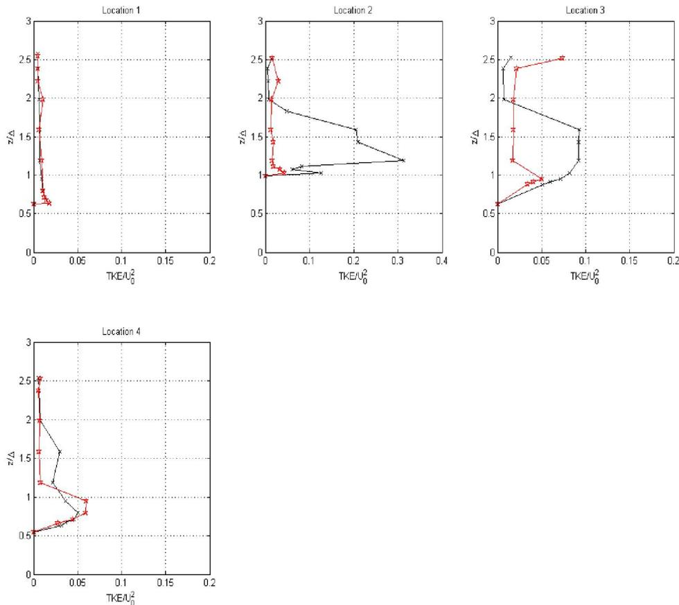
Figure 4: Comparison of turbulent kinetic energy at different locations for the vegetated and non-vegetated weir (\* (red) non-vegetated weir and x (black) vegetated weir for a leeward slope of 1:7 with  $Q=40l/\text{sec}$ ).
