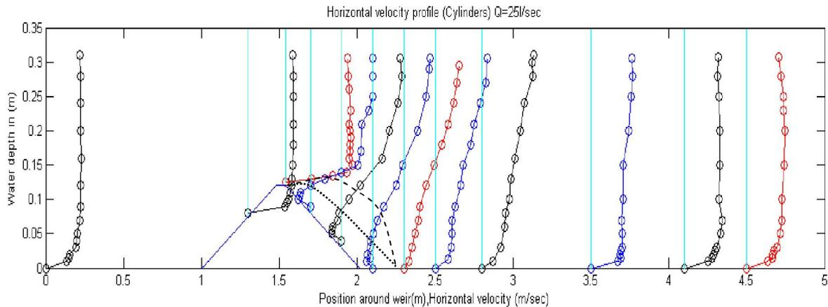
Figure 5(b): Measured horizontal velocity profiles for vegetated weir with downstream slope 1:4 (Submerged flow conditions, Froude No. = 0.25)  $Q=25$  l/sec
