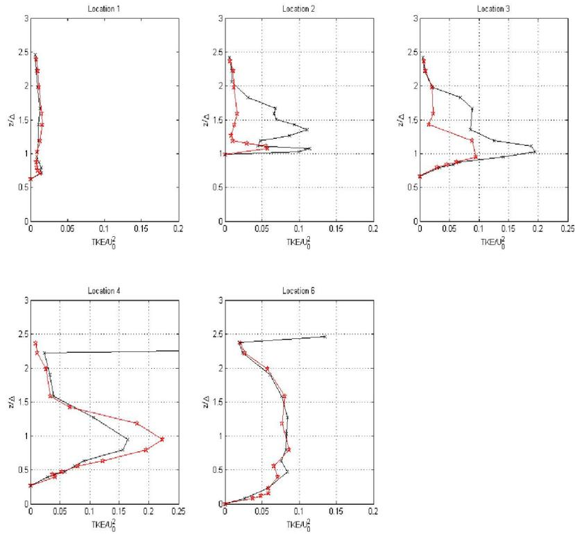
Figure 2: Comparison of turbulent kinetic energy at different locations for the vegetated and non-vegetated weir (\* (red) non-vegetated weir and x (black) vegetated weir  $Q=25$  l/sec).
