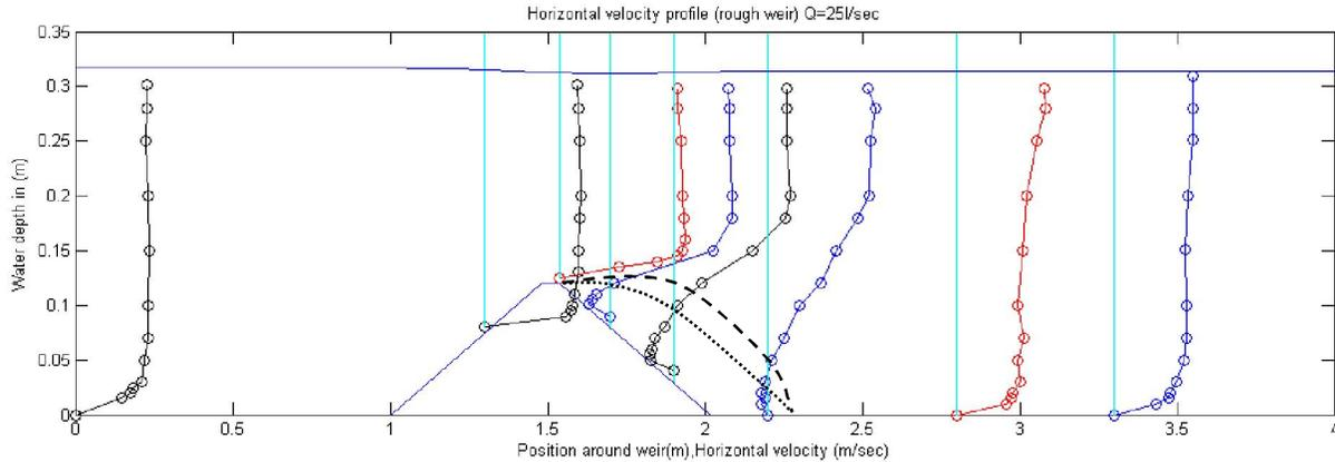
Figure 5(a): Measured horizontal velocity profiles for rough (non-vegetated) weir with downstream slope 1:4 (Submerged flow conditions, Froude No. = 0.25)  $Q=25$  l/sec
