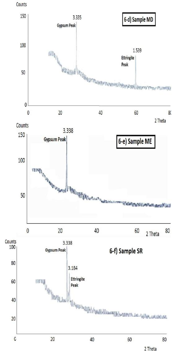
Figure 6 (a,b,c,d,e,f): XRD results of the Sulfate test showing the ettringite and gypsum formation
