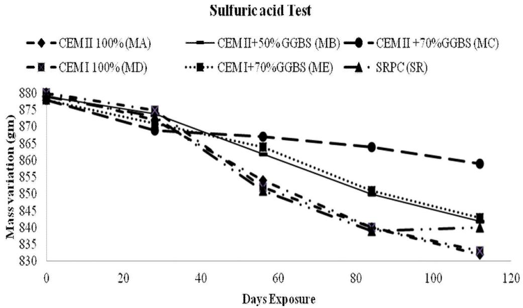
Figure 7: Mass loss of samples after sulfuric acid exposure
