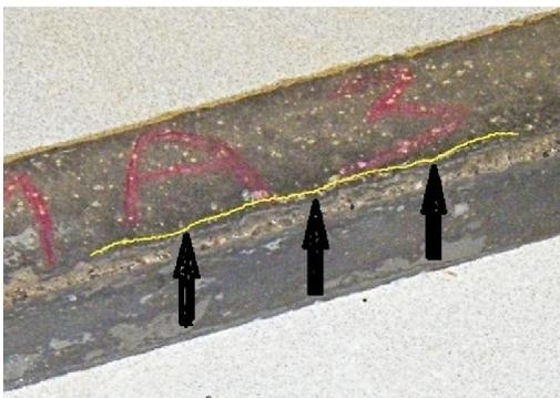
Figure 3: White filled crack in MA Specimen
