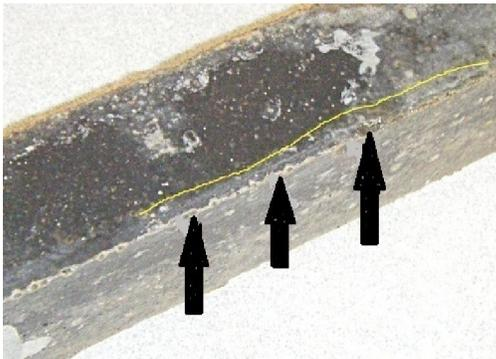
Figure.2: White filled crack in SR Specimen
