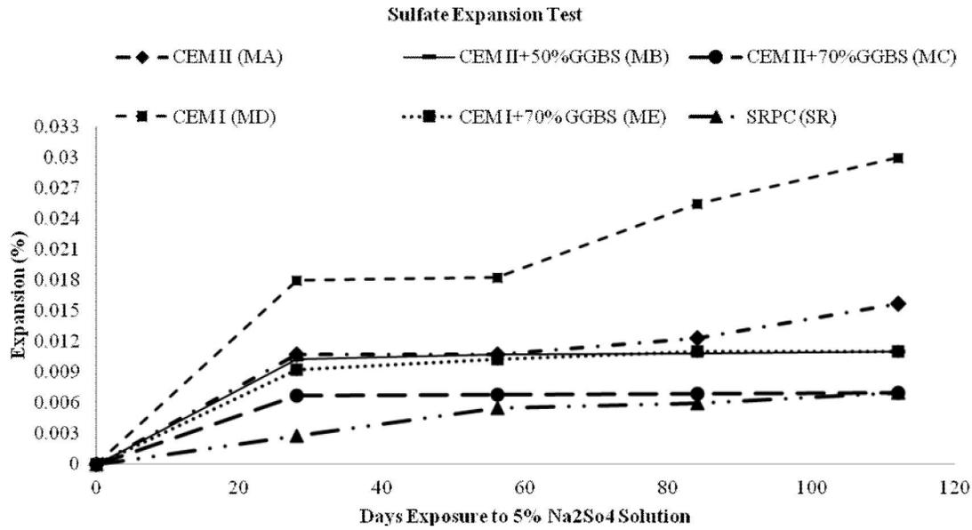
Figure 1: Results of sulfate expansion test
