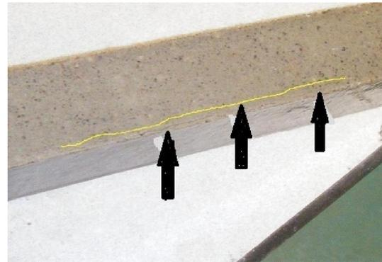
Figure 4: Longitudinal crack in ME specimen
