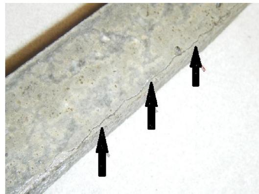
Figure5: Longitudinal crack in ME specimen
