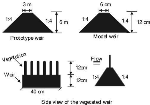
Figure 2. Prototype weir and Model weir (scaled 1:50)
