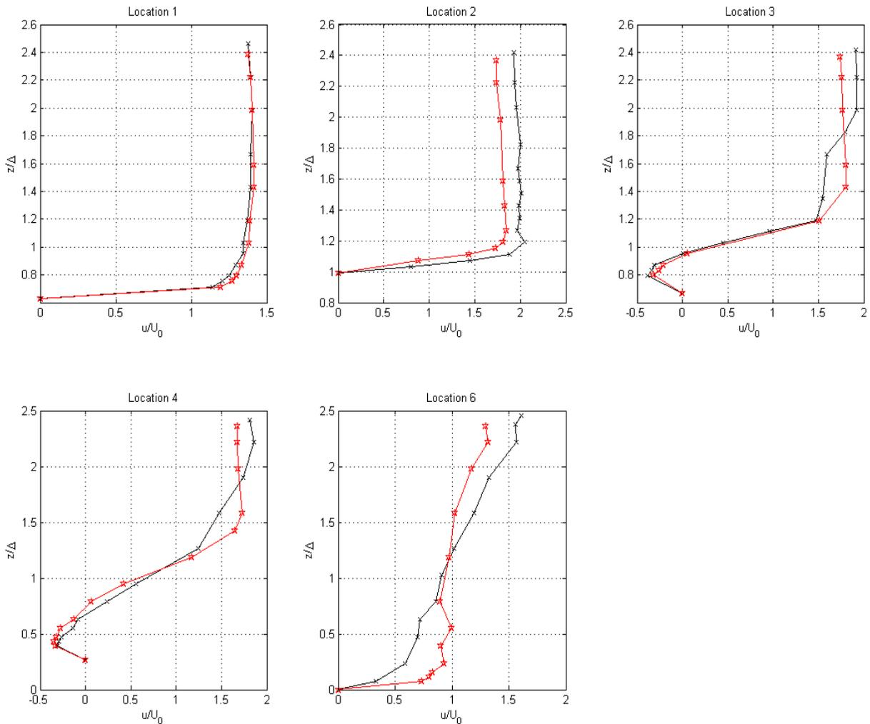
Figure 5 (a): Comparison of longitudinal velocity profiles at different locations for the vegetated and non-vegetated weir (\* (red) non-vegetated weir and x (black) vegetated weir  $Q=25$  l/sec).
