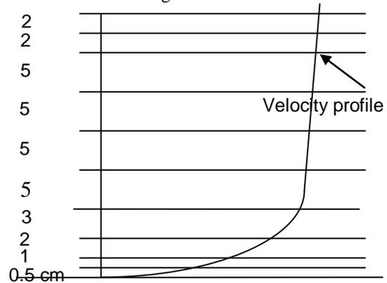
Figure 3. Vertical positions for velocity measurements at a cross-section
