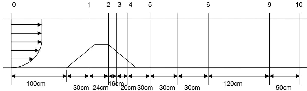
Figure 4: Cross-sectional locations for measuring velocity profiles.
