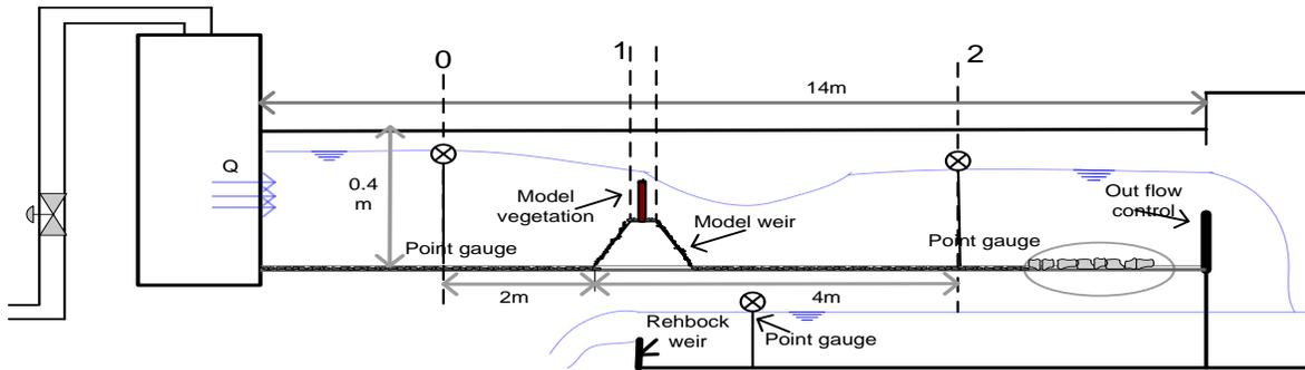
Figure 1. Experimental rectangular flume
