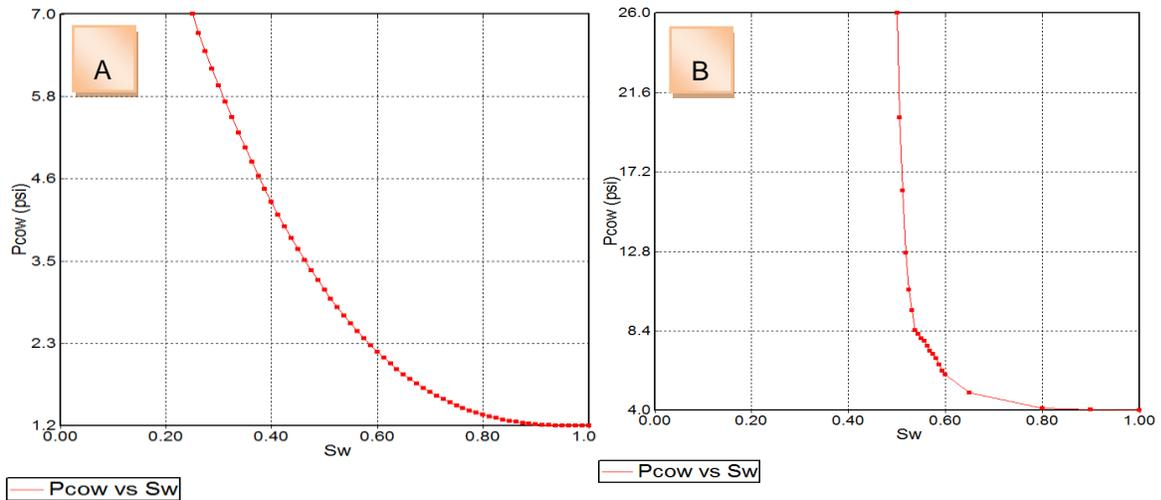
Figure-8 Capillary pressure curve for good rock and B) Capillary pressure curve for bad rock
