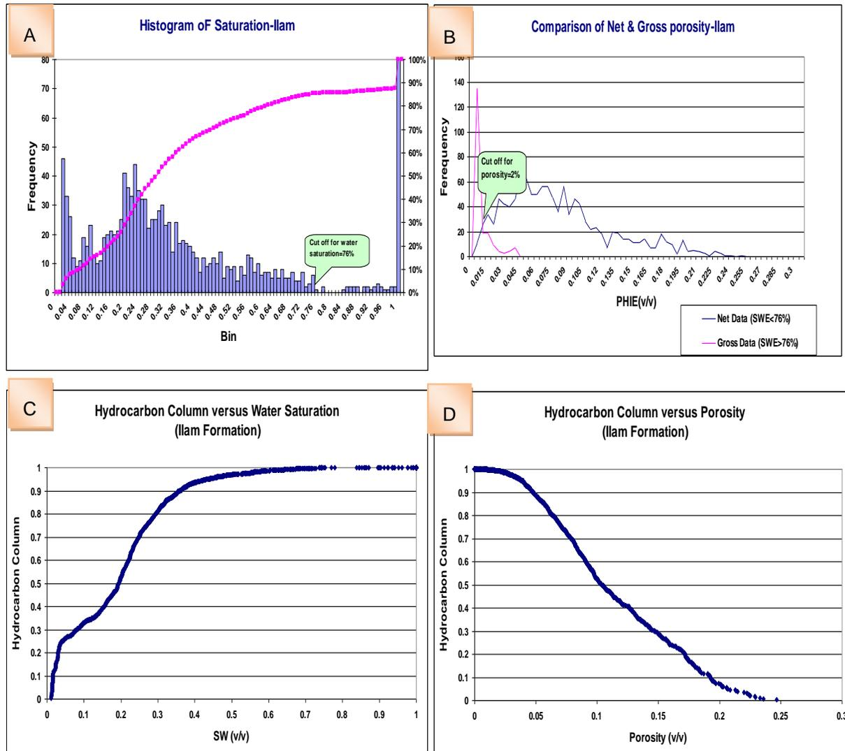
Figure-10 A) plot of water saturation distribution modality, B) categories of porosity distribution and C-D) effect of determined cut off criteria on hydrocarbon column
