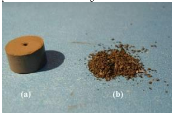
Figure6. Samples form, a) Pressed raw material b) Synthesized without pressurized environment by inert gas (under vacuumed condition or Argon gas flow) c) Synthesized in 1.9bar Argon gas pressure
