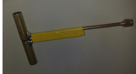
Figure 1. 1900 MHz cylindrical wire dipole antenna
