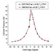
Figure 2. Peak Cylinder Pressure with respect to crank angle at equivalent ratio of 0.38 and inlet temperature of 175° C in both experimental and simulation study
