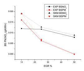
Figure 4. BSPM &  $BSNO_x$  versus EGR at three load condition in both experimental and simulation study.
