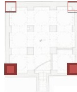
Figure 19 – The position of wind catchers in Belan water storage (Source: authors)
