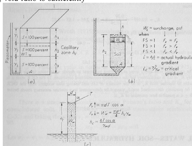
Figure 2-7 (a) Soil/water relationships for effective and pore-pressure concepts; (b) critical hydraulic gradient and concept of safety factor against a "quick" condition; (c) computation of height of capillary rise in a capillary tube.
