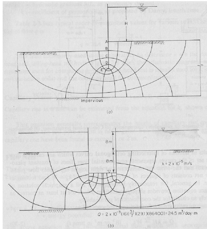
Figure 2-9 Typical flow nets as used for sheet-pile or cofferdam structures. (a) Single sheet-pile wall or other wall too far to influence net; (b) double-wall cofferdam -9§ used for bridge piers, etc.
