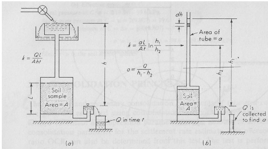
Figure 2-8 Schematic for permeability determination. (a) Constant-head permeameter; (b) falling-head permeameter.
