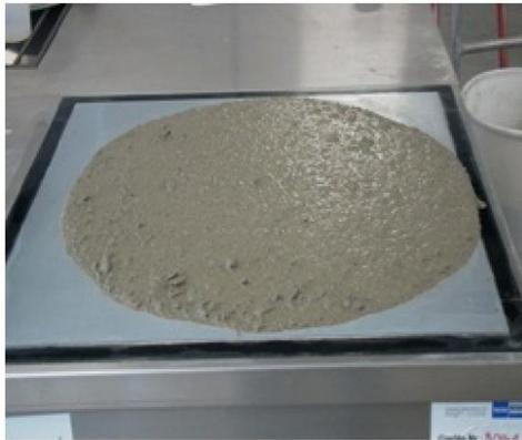
**Fig. 3. Slump flow of self compacting concrete**
