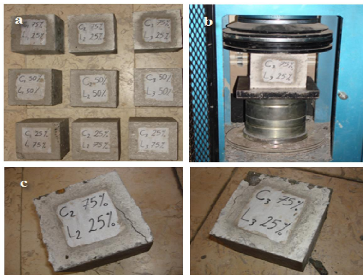
Fig. 2. (a, b, c) Testing compressive strength of concrete specimens: (a) specimens before testing, (b) Loading of specimens, (c) after testing.
