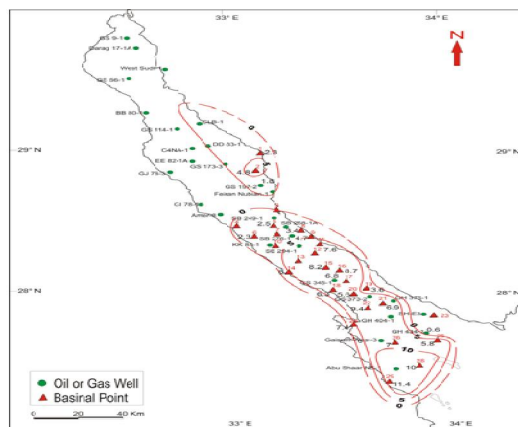
Figure 6: Time of hydrocarbon peak generation, expulsion, and migration of the Nubia Fm Gulf of Suez. Contour interval = 5 mmybp
