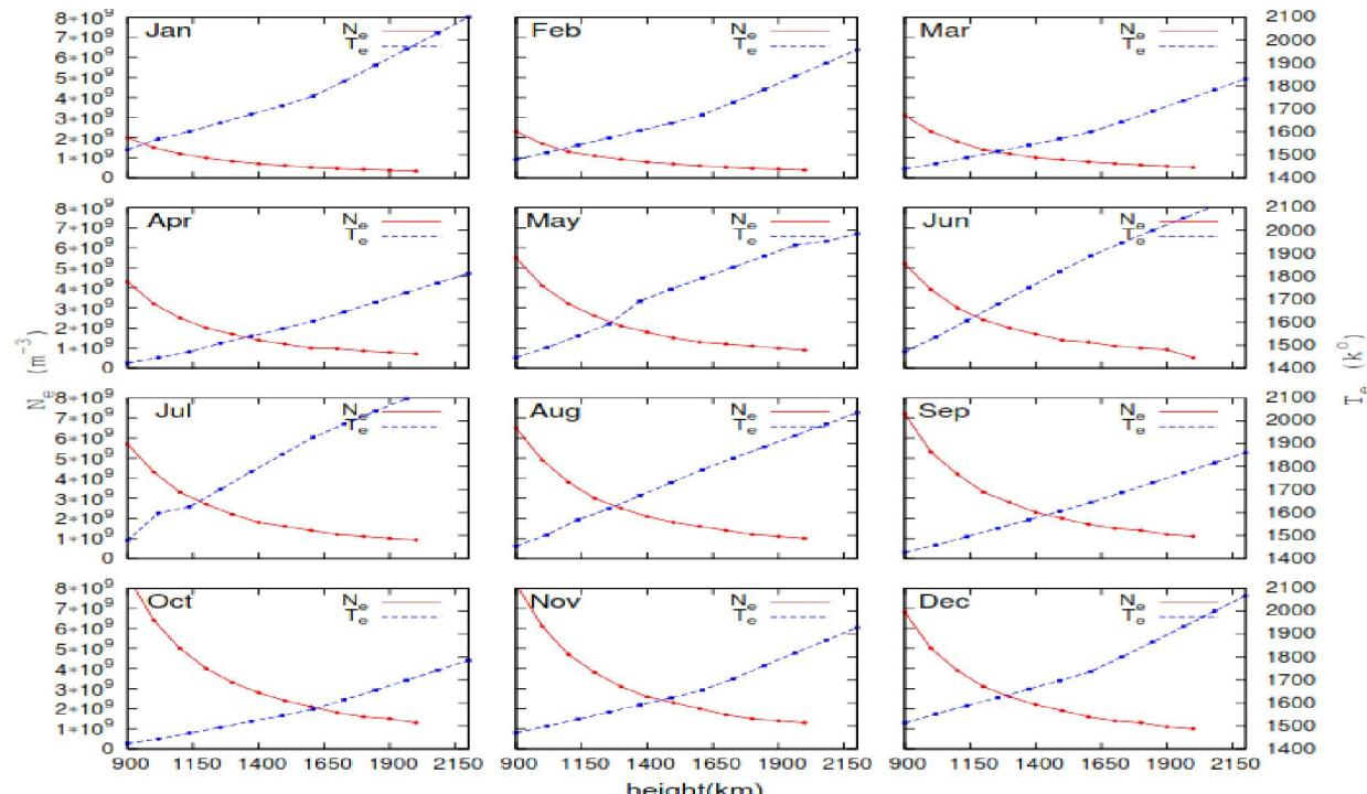
Figure 2. Annual variations of  $N_e$  and  $T_e$  in the using the IRI data topside ionosphere within the height 900km-2000km for 2011, using the IRI data
