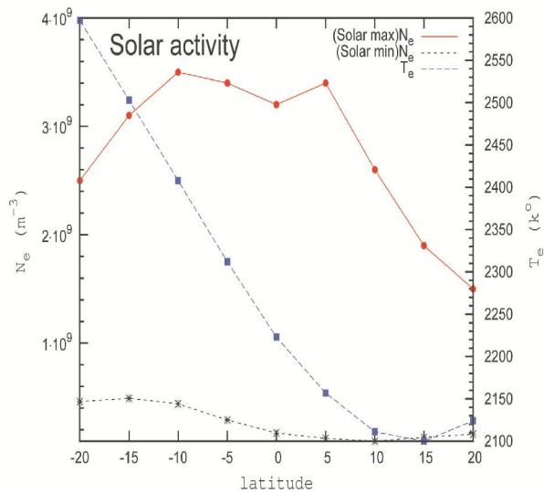
Figure 3. Solar activity variations of  $N_e$  and  $T_e$  in the topside ionosphere within  $-20^\circ - 20^\circ$  latitude for 2011, using the IRI data
