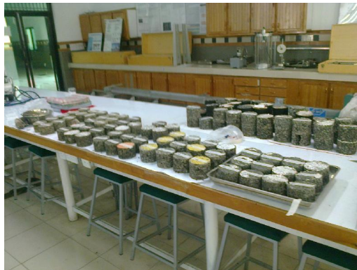
Figure 6. Laboratory Marshall Samples
