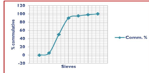
Figure 3: Gradation of the Cold Recycled Mixes
