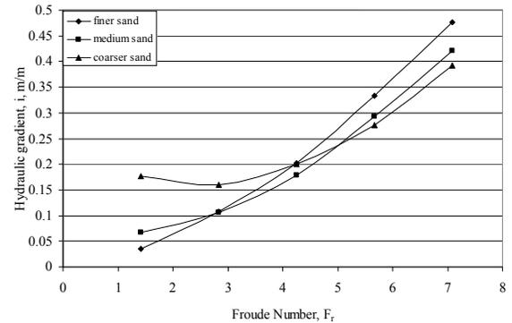
Fig. 6 Hydraulic gradient for PVC pipe and 10 % sand concentration for different sands
