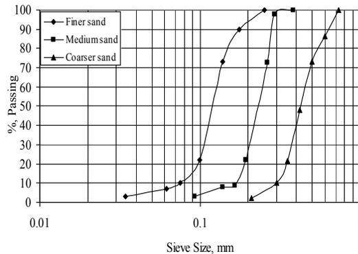
Fig. 2 Grain size distribution of different sands used in the present paper
