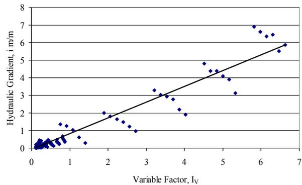
Fig. 10 Hydraulic gradient variations with the affecting variables
