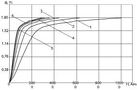
Figure 6. - Changing of magnetization curve of sample's material B(H) in order to provide in the model dependency of  $[PHI]_{ta_max}(i_{max})$  corresponding to the experimental  $[PHI]_{ta_max}$   $e_x(i_{max} e_x)$ : 1,2,3,4,5 - curves in the process of approximation, 6- resulting (or 'recovered') characteristic of the material.
