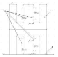
Figure 4 – 2D-model of magnetic system: 1 - magnetic conductor, magnetizing coils, 3 tested item.
