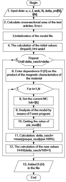
Figure 5 - Algorithm of recovering of magnetic characteristic of the item's material in accordance with method of experimental and simulation method.
