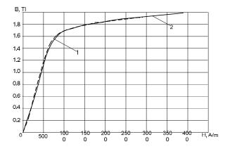
Figure 8 - Measured magnetization curves: 1 - obtained by means of proposed IMS, 2 - of a sample.
