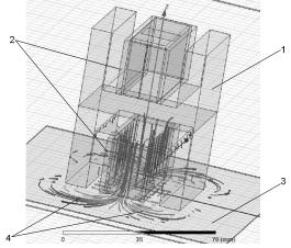
Figure 3 - 3D model of magnetic system. 1 - magnetic conductor, magnetizing coils, 3 tested item, 4 - lines of magnetic flow.
