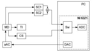
Figure 2 - Structural diagram of information and measurement system for identification of magnetization curve of sheet electrical steel.
