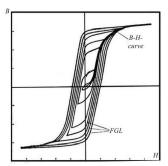
Figure 1 - Defining of magnetization curve: B-H-curve - magnetization curve, FGL – family of hysteresis loops
