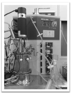
Figure 2.1: Operational configuration of the New Bruswick BioFlo 3000 STR during batch fermentation of X. campestris ATCC 13951.
