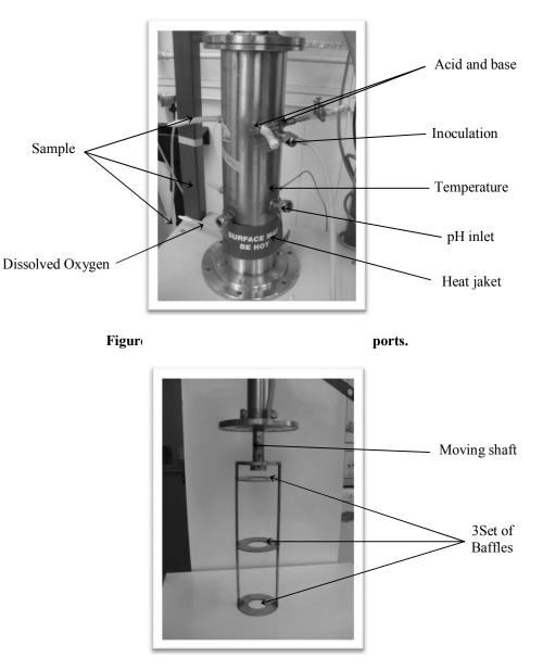
Figure 2.3: A set of three orifice baffles and the supporter
