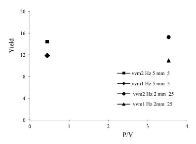
Figure 3.3: shows the power density of different agitation rates used in this study of STR vs. the yield after 96 hours.
