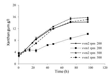
Figure 3.2: The Effect of the interaction between aeration and agitation speed on xanthan gum production in batch cultures of X. campestris ATCC 13951 in the STR at 30 °C.
