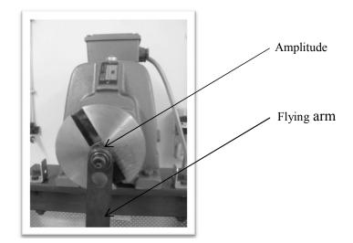
Figure 2.4: The motor and the adjustable amplitude
