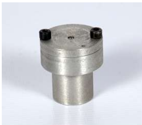
Fig. 1: The custom made apparatus used for shear punch testing.
