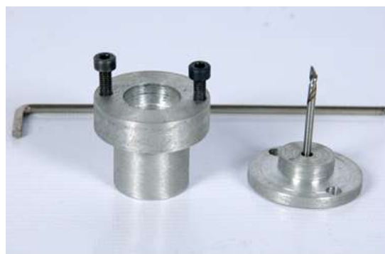
Fig. 2: The apparatus opened showing the two sections: the upper one having the tool steel punch inserted through the punch hole.
