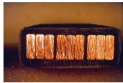
Figure 1. Cross-section of a three-turn coil made with an epoxy mica paper insulation system [3].
