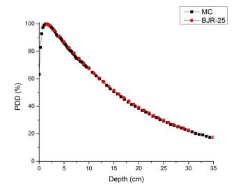
Figure 2: The PDD curves of the conventional 6 MV Varian linac beam simulated (squares) and obtained from BJR-suplement-25 (circles) for a  $10 \times 10$  cm<sup>2</sup> field-size in a water phantom.
