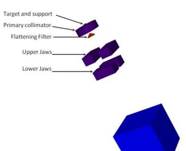
Figure 1: The simulated geometry of the conventional 6 MV Varian Clinac 2100C.
