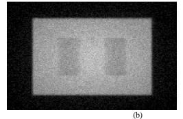
Figure 5: The acquired images of two cylindrical bones with 2 cm diameter placed inside water phantom with 5 cm thickness at 100 cm from the target by (a) the conventional beam and (b) the copper target beam.
