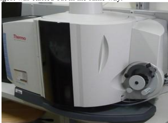
Figure 1: Biological samples preparation for determination of trace elements using inductively Coupled Plasma/ Emission Spectrometer (ICP/ES)
