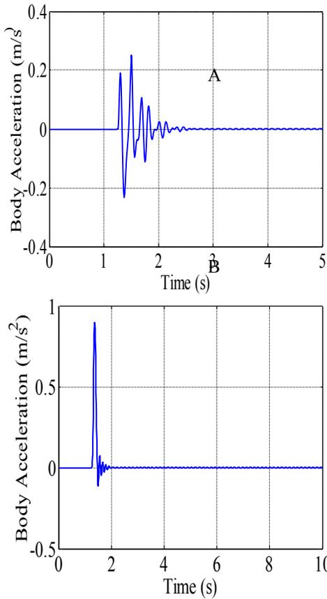
Figure 8- The acceleration on car body. (A) Active (B) Passive
