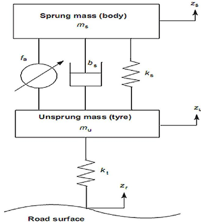
Figure 1: An active suspension system model
