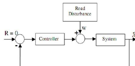
Figure 4- Closed Loop System
