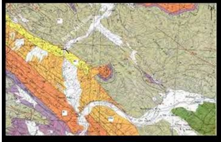
Fig. 3 The site of Jere dam in geology map of the region (black arc) As, Gs, Mn, Lb, Aj, Bk show Bakhtiary formation, Aghajari, Mishan, Lahbari, Gachsaran and Asmari, respectively[5].
