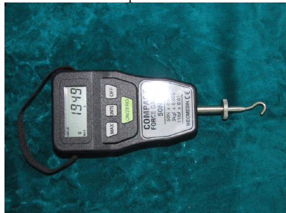
Fig (7) Force gauge was used to record the retention.
