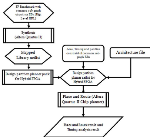
Figure 4: Design flow for common subgraph EBs using Altera Quartus II
