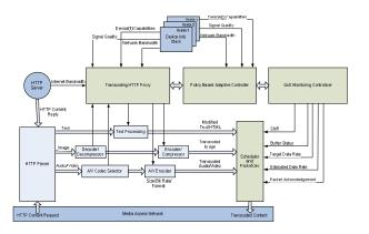
Fig. 2. Adaptive Transcoding Proxy Gateway Architecture
