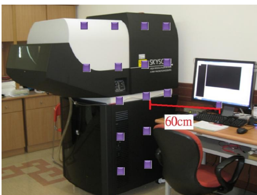
Figure 3 (a) The positions of TLD on the right side of instrument surface. (b) The positions of TLD on the left side of instrument surface and control console.
