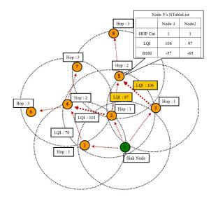
We developed the reliable multi-hop routing protocol based on the tree structure to retain seamless network connection. It was implemented with the gradient flooding mechanism, and based on TinyOS2.0. It adaptively selects the paths to relay data throughout the networks by the analysis of present multiple link qualities. To setup paths, it uses index that has hop count from the destination node and link quality metrics including LQI and RSSI.
