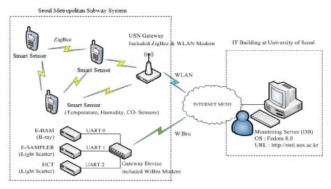
Fig. 1 EAPMS System Configuration
