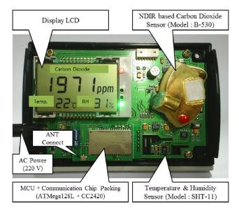
Fig. 2 Smart Sensor Prototype
