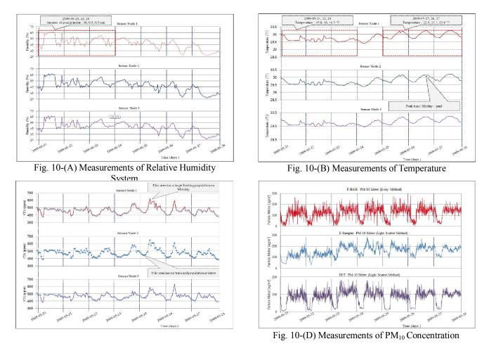
Fig. 10 Remote Measurements from Smart Sensors in Underground Subway System
