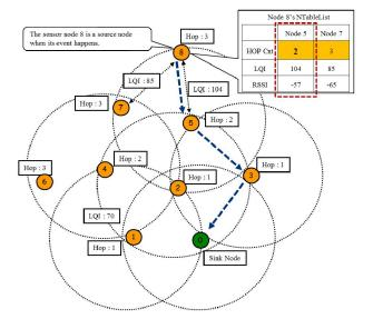
Fig. 5 Data Delivery Phase using Hop Count Priority
