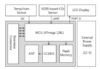
Fig. 3 Block Diagram of Smart Sensor
