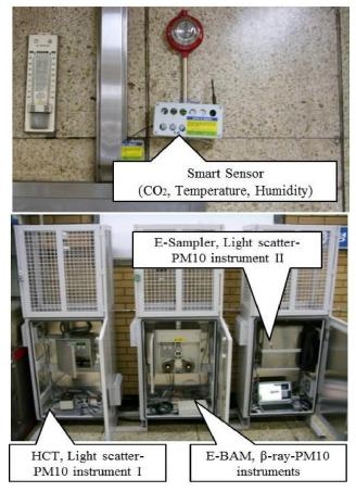
Fig. 9 EAPMS Pilot Project Setup in Subway System
